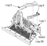
Figure 31 - Installing Logs 5 and 6
